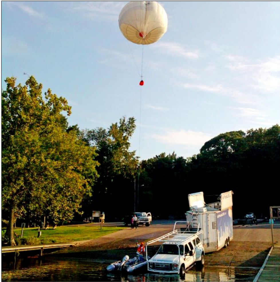
Tethered surveillance balloon is transferred from the mobile launch trailer to a patrol boat.
